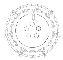
4) Attach inside hook first. Pull chain tight and attach as close to first cross chain as possible.
