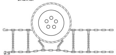
3) Drive your vehicle over the chains, so that the tire is resting between the spread cross chains. Pull chain up and around tire. Make sure chain is centered on tire.
