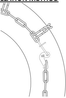
5) To install outside fasteners, pull chain tight and slip a link as close the first cross chain as possible over the fastener.
