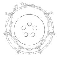
3) Rotate tire ¼ - ½ turn, so that gap in chain is towards top of tire
