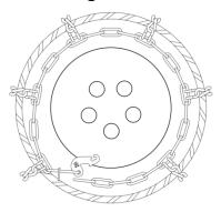
2) Drape chain over tire, making sure chain is centered on tread face of tire. Pull the ends of the chain at the bottom of the tire towards each other
