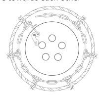
3) Rotate tire ¼ - ½ turn, so that gap in chain is towards top of tire
