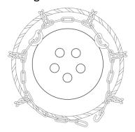
2) Drape chain over wheel, keeping chain centered on tire. Pull two ends of chain towards each other at the bottom of the tire.
