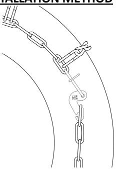
5) To install outside fasteners, pull chain tight and slip a side chain link as close the first cross chain as possible over the fastener.
