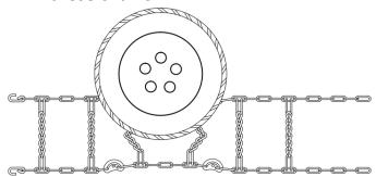
3) Drive your vehicle over the chains, so that the tire is resting between the spread cross chains. Pull chains up and around tire. Make sure the chain is centered on the tire
