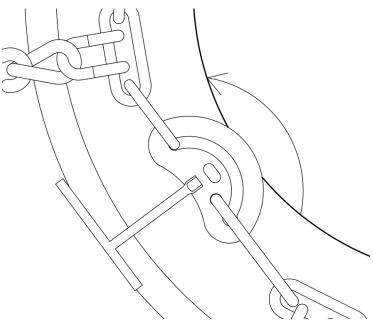
5) To tighten the cams, insert T handle into slot, and turn counter clockwise so the connecting link can move through the channel.
