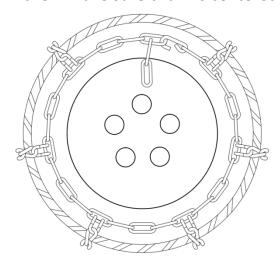
4) Attach inside quick hook on back of tire first. Pull chain tight and attach as close to first cross chain as possible.
