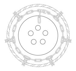
4) Attach inside quick hook on back of tire first. Pull chain tight and attach as close to first cross chain as possible. Repeat this process for the outside fastener.
